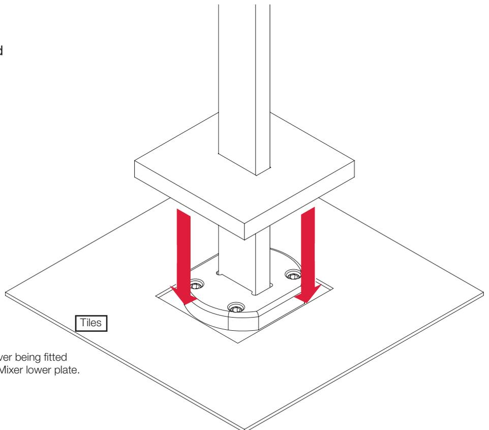
Fig. O. Base cover being fitted over Bath Filler Mixer lower plate.
