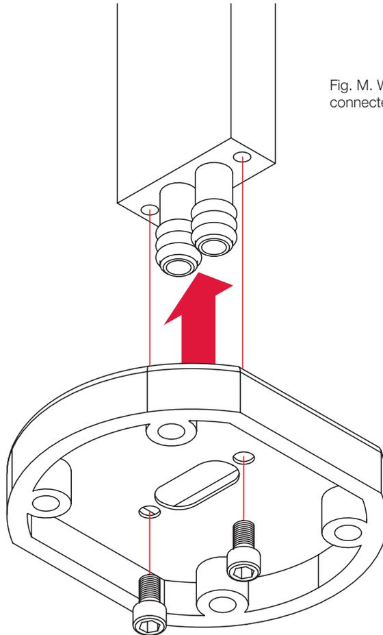
Fig. M. Water feed tubes being connected to base.
