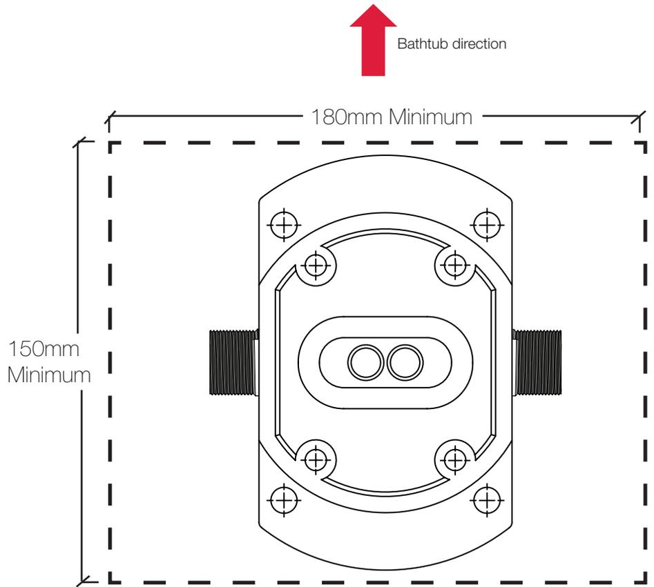
**Please note:** The depth of the floor pit will dictate the overall height of the Bath Filler once installed. The bottom plate of the Bath Filler body may sit on or underneath the tiled floor surface, but the base must remain underneath.
