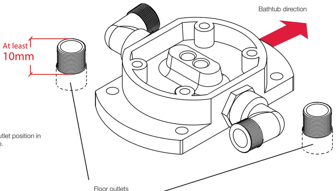
Fig. G. Floor outlet position in relation to base.
