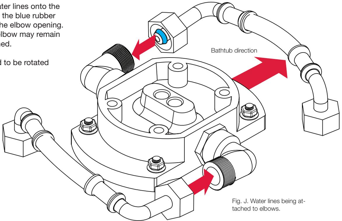
Fig. J. Water lines being attached to elbows.
