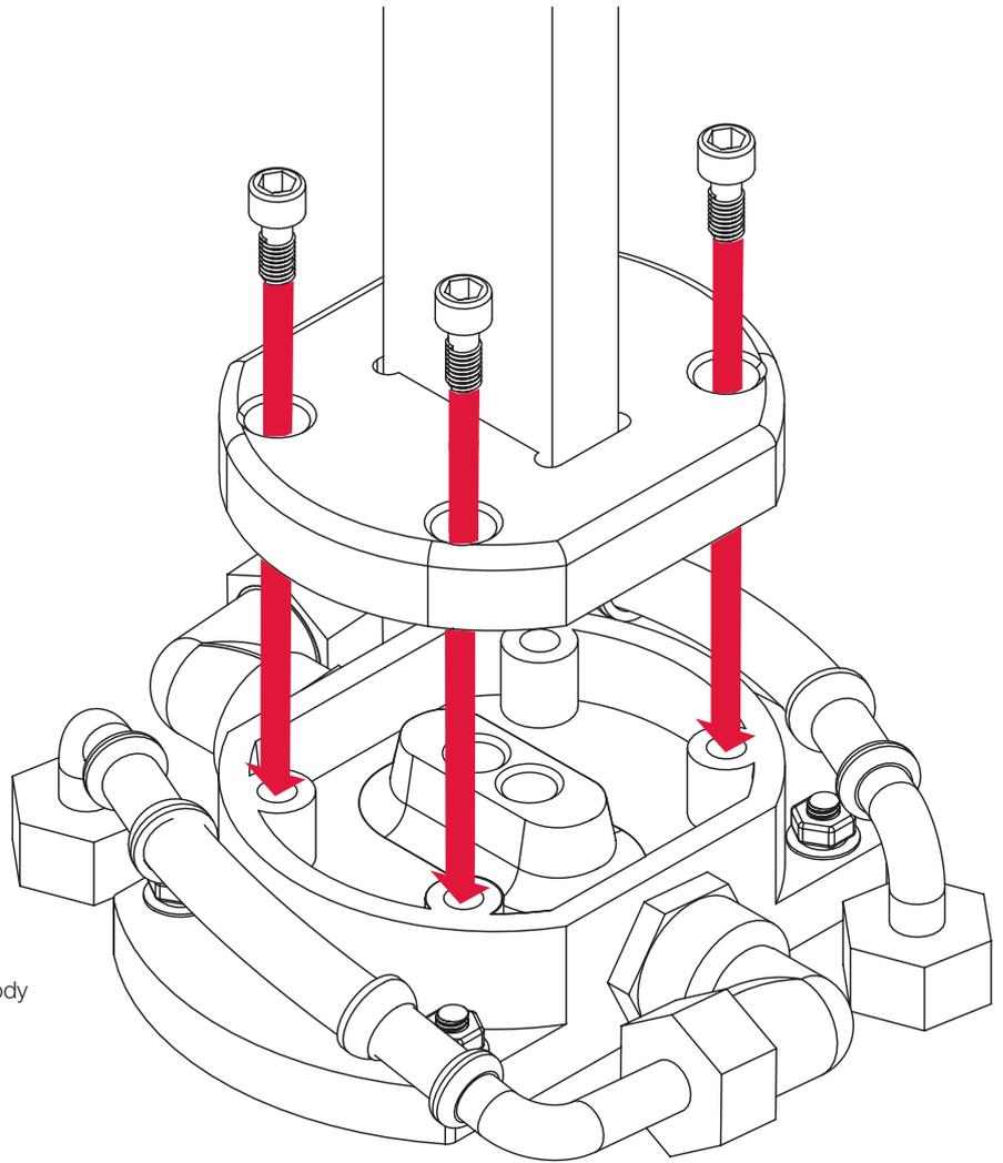
Fig. N. Base mounting screws connecting Bath Filler Mixer body to base.
