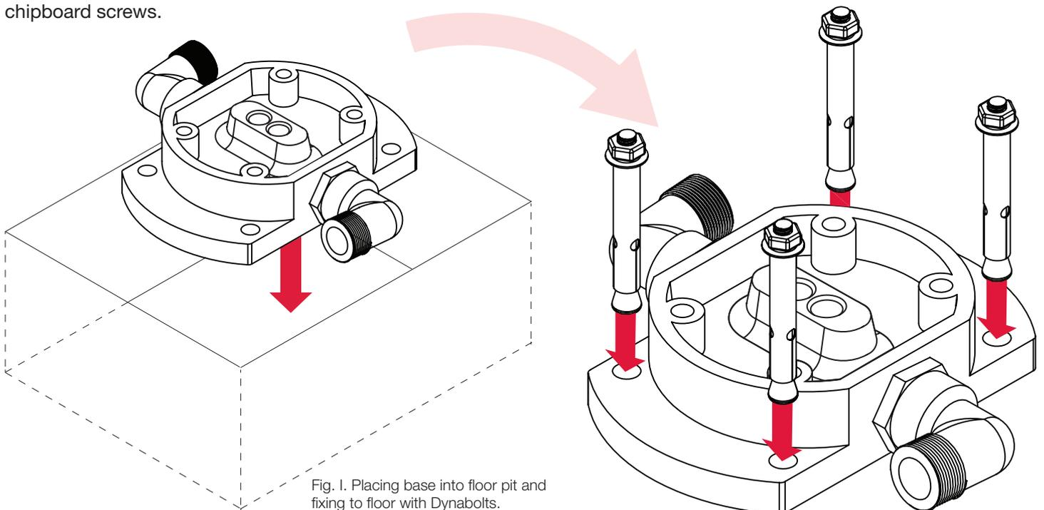
Fig. I. Placing base into floor pit and fixing to floor with Dynabolts.
