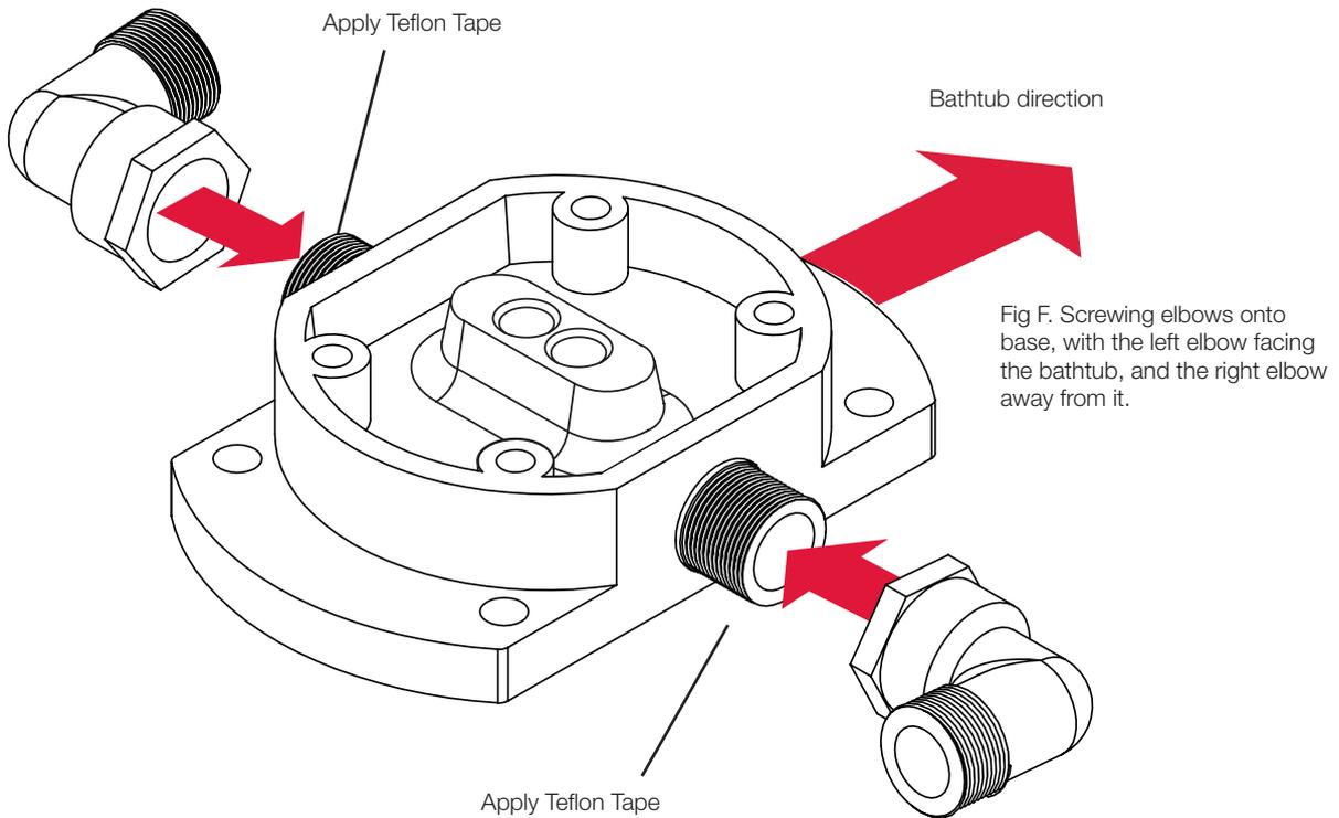
Fig F. Screwing elbows onto base, with the left elbow facing the bathtub, and the right elbow away from it.
