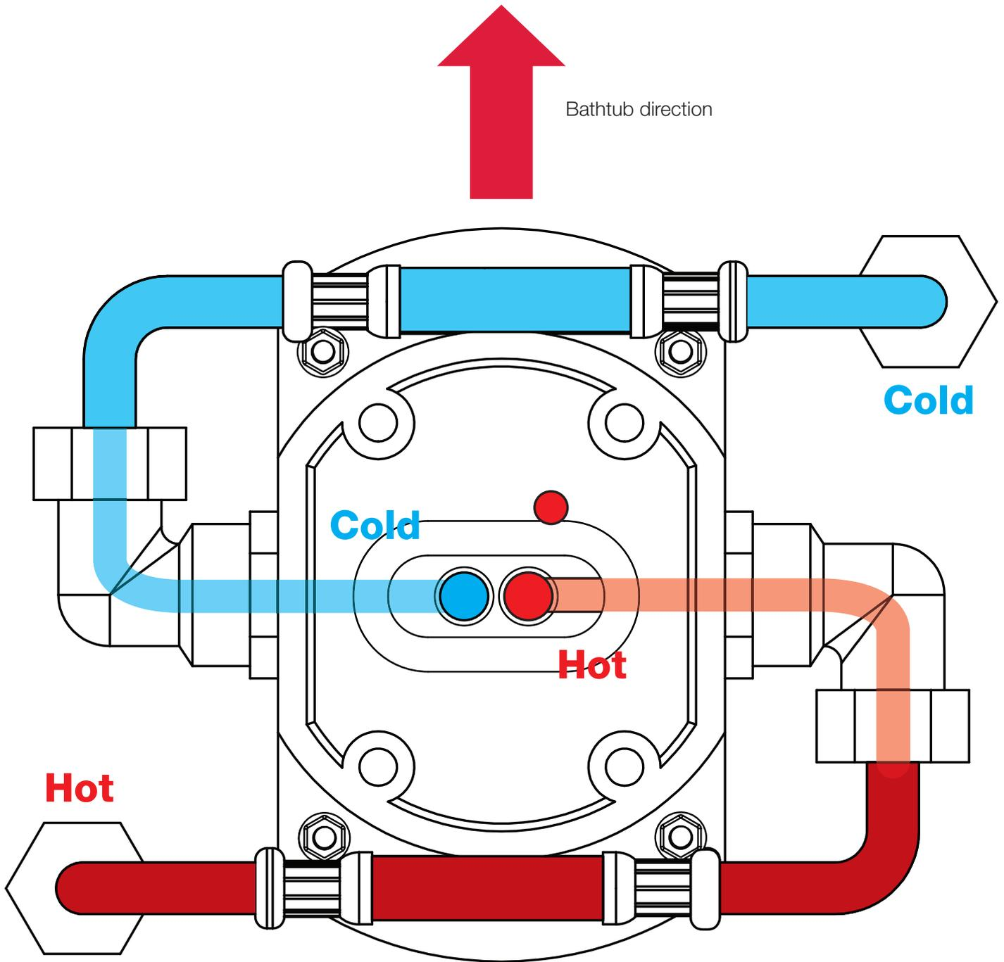
Fig. L. Layout of hot and cold water lines.
